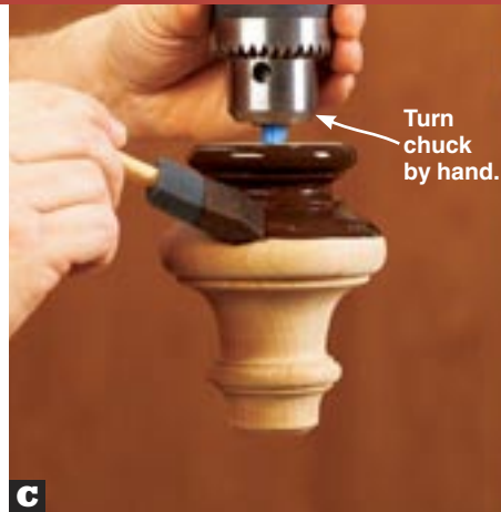
C Turning the drill-press chuck by hand, apply stain with a brush. Then remove most of the excess stain with a paper towel.
