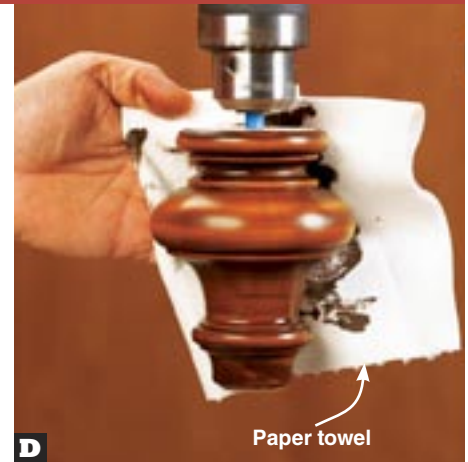
D With the drill press running, use a paper towel to finish wiping the stain. Remove the feet from the chuck and set them aside to dry.
