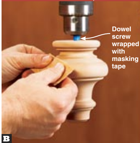
B With the drill press running at 450 rpm, sand the feet with a progression of 120-, 150-, and 220-grit sandpaper.
