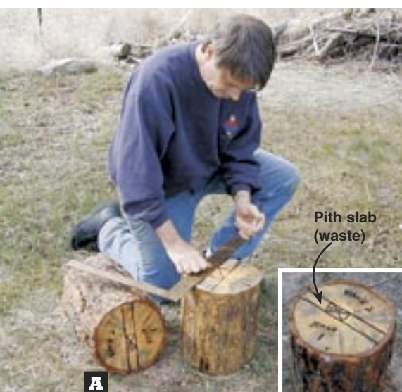
A To remove the pith and a large-diameter unstable zone around it, draw lines with a permanent marker to guide your cuts. The slab marked here is about 1¼" wide.
